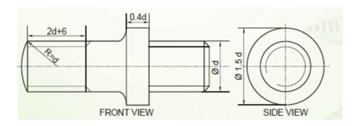
6. ( Hint : Free hand sketch of flat head rivet ,stand dimensions calculated with  $d=20\ mm$  ).
