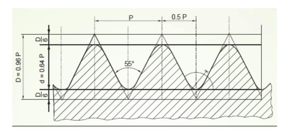
3.( Hint : Standard dimensions of Metric thread internal should be calculated with the pitch given = 60 mm)
