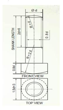
5. (Hint: Free hand sketch of stud with collar, d can be taken proportionately and calculate standard dimensions).
